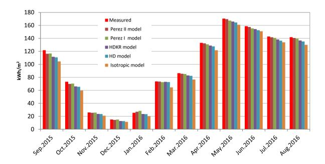
Fig.7. Calculated and measured total radiation on 50° tilted south facing surface (Sep.2015 – Aug.2016) [29]
