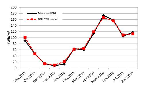
Fig.8. Calculated DNI (DTU) and measured DNI in the Tars solar heating plant. [29]
