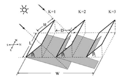
Fig. 10. Internal shading for collectors within an array [30]
