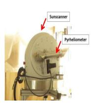
Fig.4. Used weather station and pyrheliometer of the Tars solar heating plant [29]
