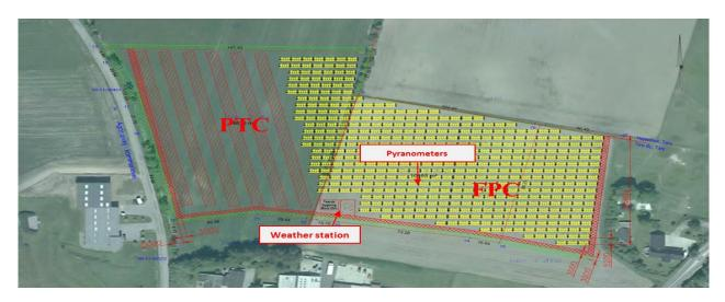
Fig.2. Location of the weather station and pyranometers (PTC: parabolic trough collector, FPC: flat plate collector) [17]
