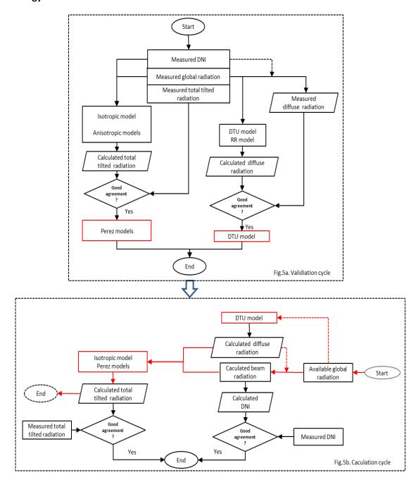
Fig.5.Schematic illustration of the methodology (Fig.5a.Validation cycle, Fig.5b.Caculation cycle). [29]
