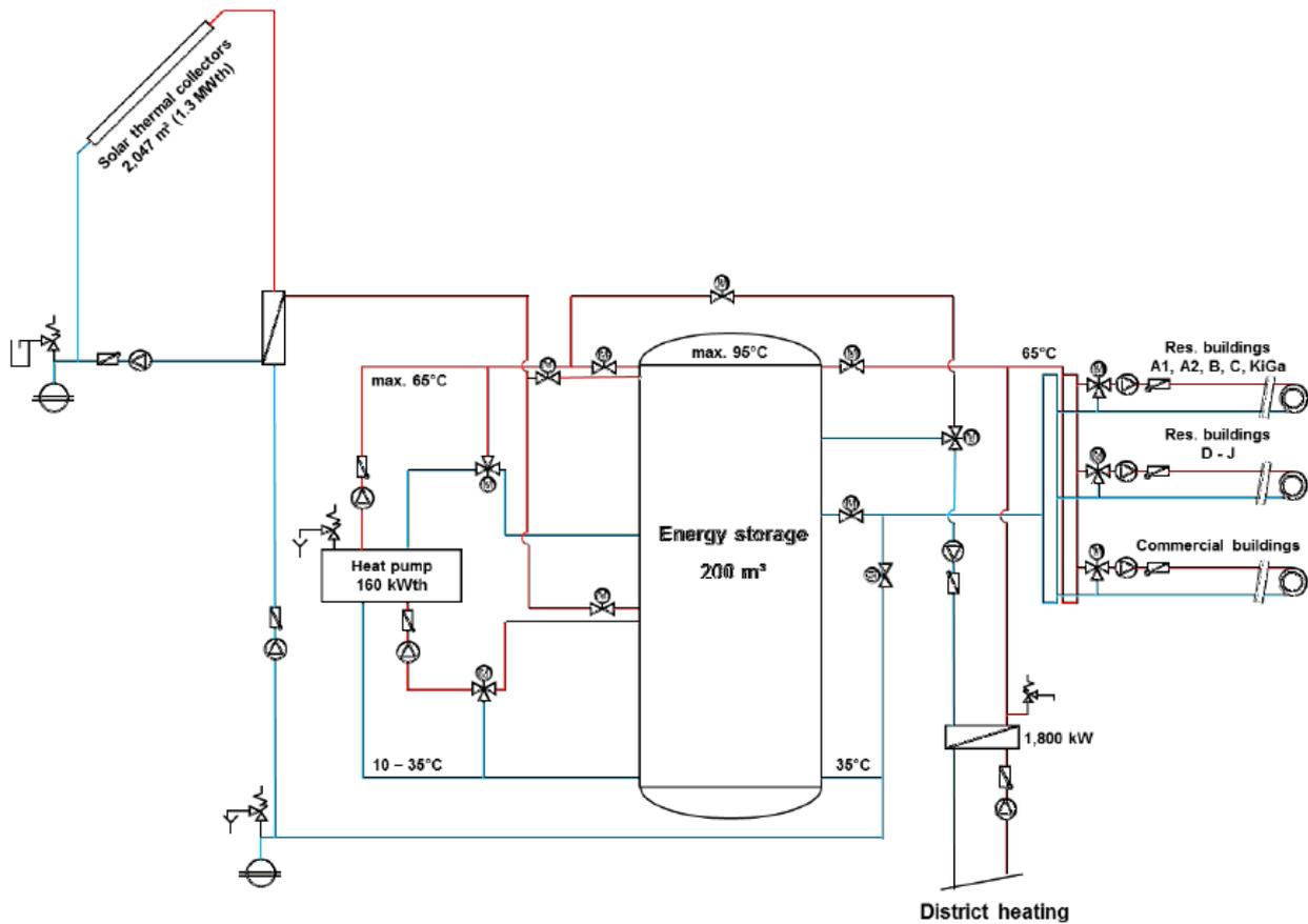
Figure 11. Hydraulic scheme of the heat supply system in Salzburg-Lehen (Source: AEE INTEC)
