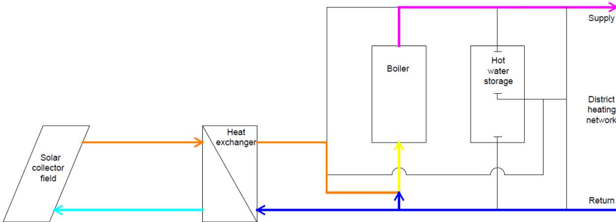
Figure 3. Integration of ST as boiler preheater
