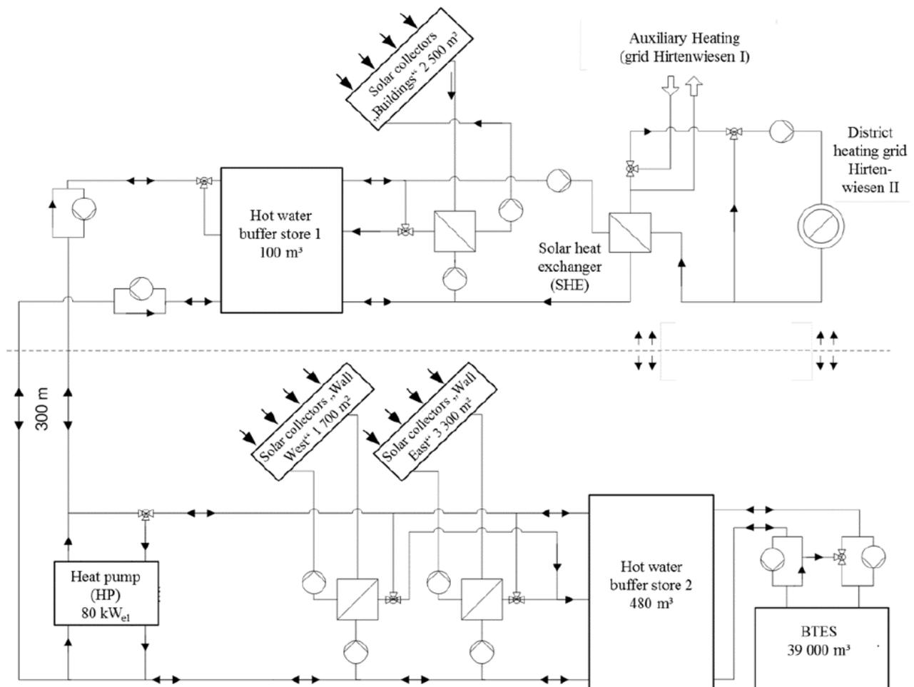
Figure 9. Hydraulic scheme of the SDH system in Crailsheim (Source: [3])
