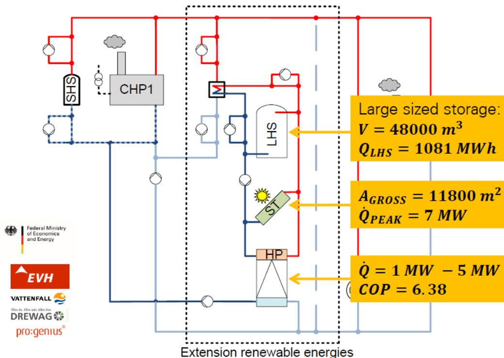
Figure 12. Concept for integration of ST and heat pump in an existing DH system (Source: [4])
