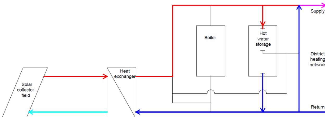
Figure 6. Integration of ST with return as shunt
