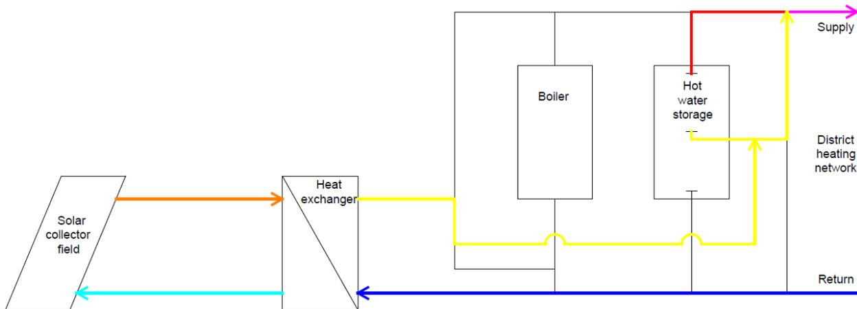
Figure 4. Integration of ST in combination with hot-water storage
