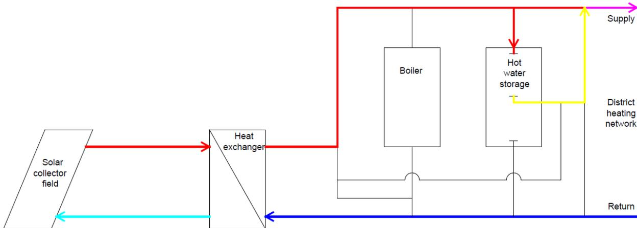
Figure 5. Integration of ST with storage as shunt
