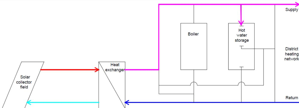
Figure 1. Return-to-supply integration of ST
