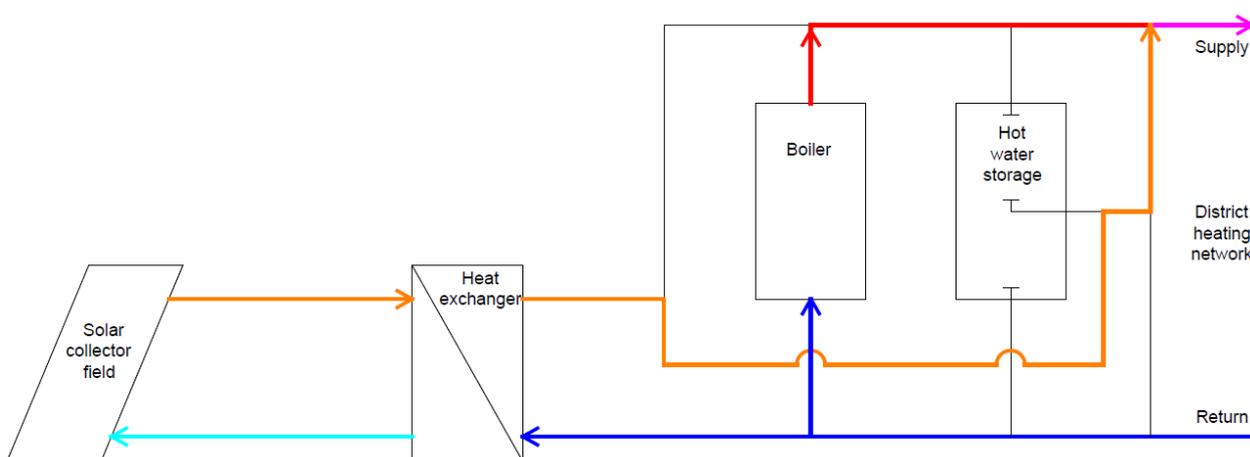
Figure 2. Indirect return-to-supply integration of ST
