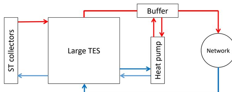
Figure 7. General integration scheme of ST with large TES and heat pump
