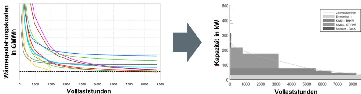
Figure 6. - left: Full load hours of the relevant generation technologies depending on the heat production costs, right: Use of an optimization tool (here VarOpt VarOpt2)) to create producer portfolios.
