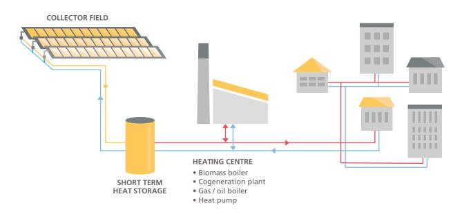
SDH is a large field of solar thermal collectors supplying solar energy to the heat network of a neighbourhood, a village or a town. This field is supplemented by a heating centre, which provides additional energy to meet all the heating needs of connected residential, public or office buildings. The heat network can likewise be supplied with surplus energy of collectors installed on the roofs of those buildings.
